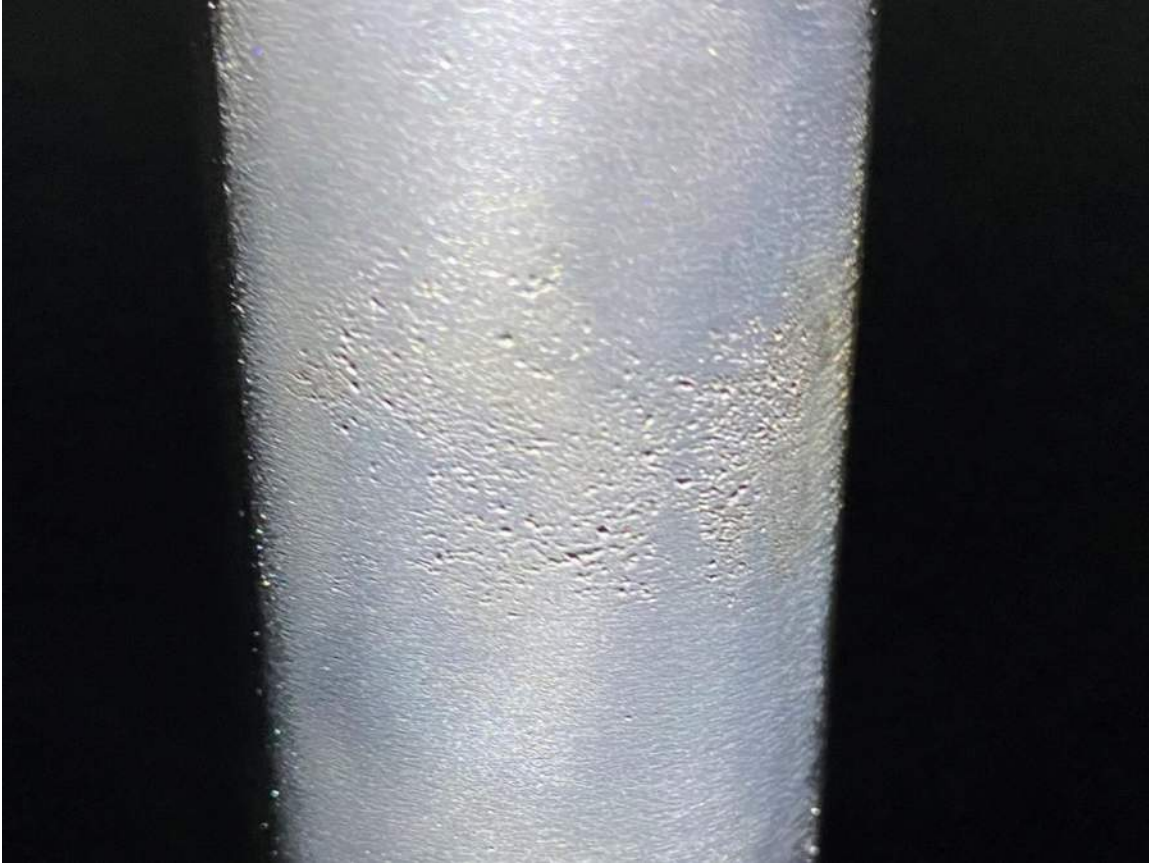
Severity level 1, mild pitting (new rod)
