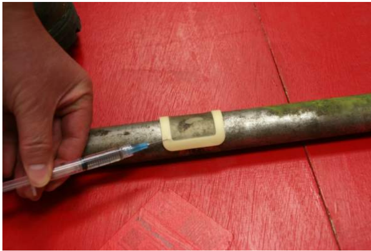
Figure 6. Photo. Injection of fluid into Bresle patch.
