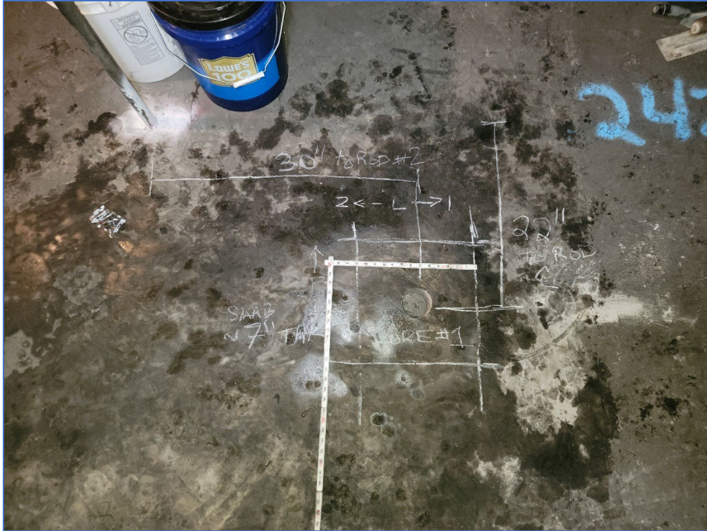
Photo 3: Typical sample hole after core extraction (Core 1 shown).
