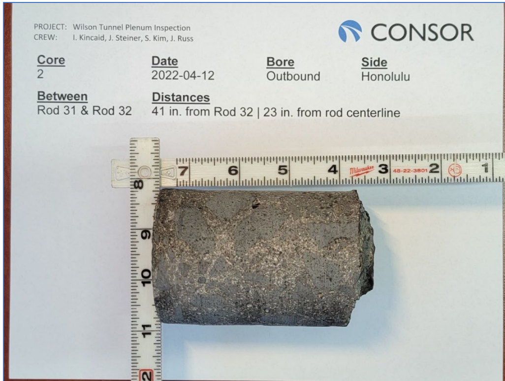
Photo 7: Core 2 after extraction.
