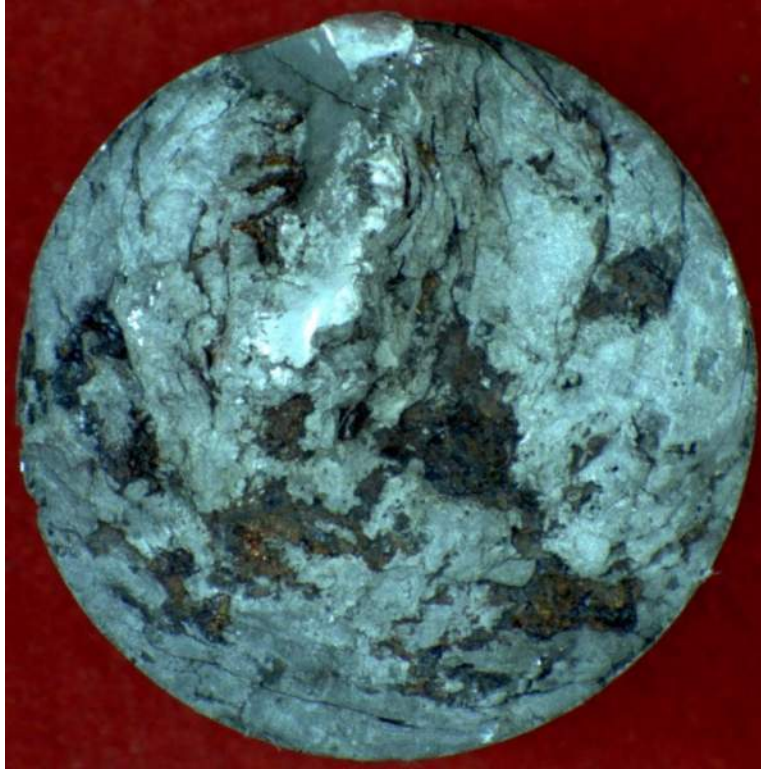
Figure 14. Photo. Rod 1 fracture surface after cleaning.
