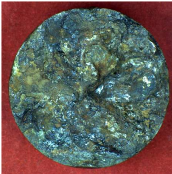
Figure 5. Photo. Rod 2 fracture surface.
